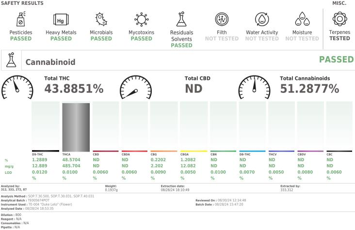
Full spectrum cannabinoid analysis utilizing High Performance Liquid Chromatography with Photo Diode Array detector (HPLC-PDA) for analysis. (Methods: SOP.T.30.500 for sample homogenization, SOP.T.30.031 for sample prep, SOP.T.40.031 for analysis on Shimadzu IC-20X0 series HPICs). Potency results for cannabis flower products are reported on an "as received" havis, without moisture correction.
